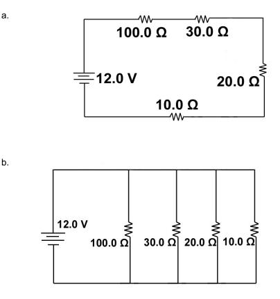
3. Find the: (a) total current, (b) total resistance, (c) power dissipated by R<sub>4</sub>.
